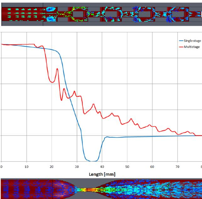
*Pressure drop comparison between single stage and multistage multipath Limiphon trim on liquid service*
